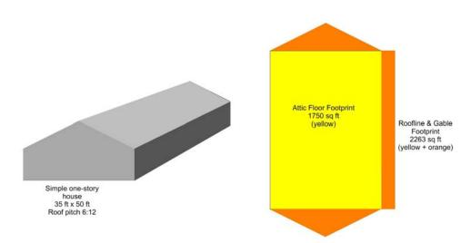
Figure 2: Comparative insulated areas for vented and unvented attic
